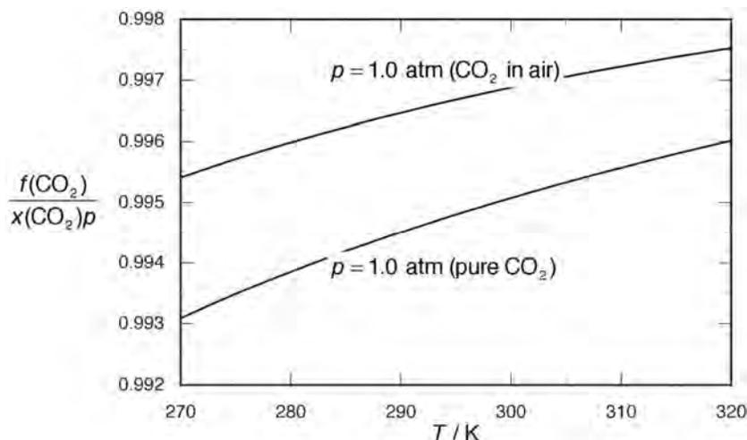
**Fig. 1** Variation of the fugacity coefficient with temperature at 1 atm total pressure for pure CO<sub>2</sub> gas and for CO<sub>2</sub> in air:  $x(\text{CO}_2) = 350 \times 10^{-6}$  (calculated using the procedure described in SOP 24 of this Guide).
