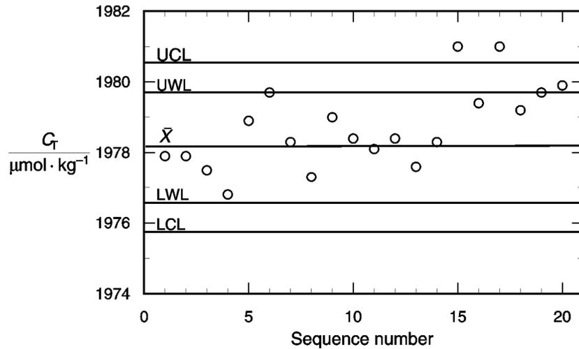
**Fig. 1** Example of a property control chart showing a trend in the data with time; control limits were calculated from the first 12 points. This chart indicates that the measurement process is not in control.
