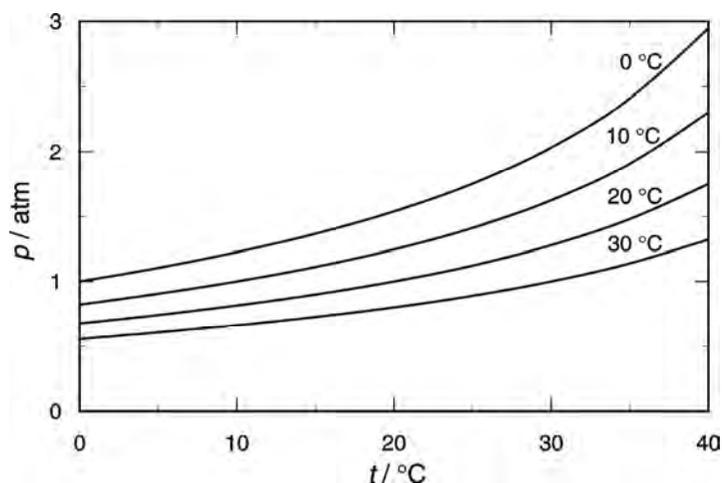
**Fig. 1** Pressure in headspace with  $r = 0.01$  as a function of temperature for various initial temperatures. In calculating this, it was assumed that the gases— $N_2$ ,  $O_2$ , Ar,  $H_2O$ —were initially at solubility equilibrium with sea water at the starting temperature, that they behaved ideally and that the initial pressure in the bottle at the indicated temperature was 1 atm.
